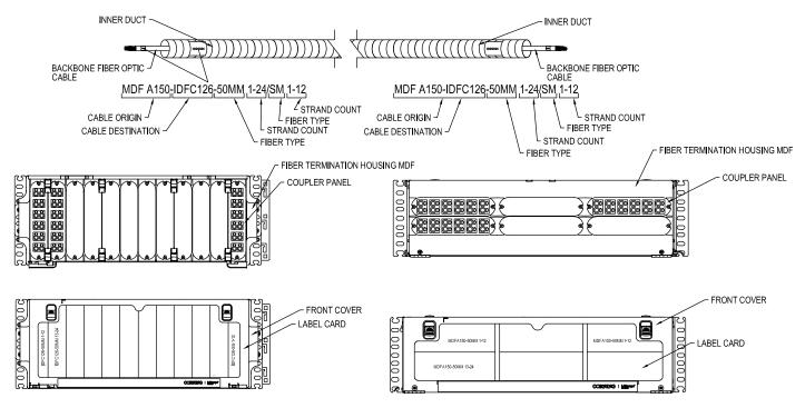
NOTE: 1) CABLE AND INNERDUCT SHALL HAVE IDENTICAL LABEL AT BOTH ENDS
