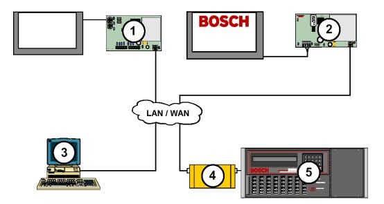
C. Data communication transmission shall use the owners existing LAN/WAN data networks with the owners existing PBX system as Alternate communications.
