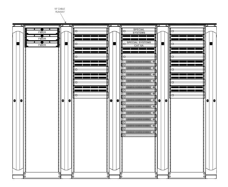
NOTE: 1. SPECIAL SYSTEM SECURITY, BMS, AV, CAMERAS, HVAC, FIRE ALARM, DIGITAL SIGNAGE 2. SPECIAL SYSTEM CAT 6A WAPS, UPLINK
