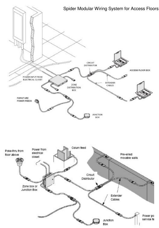
Spider Modular Wiring System for Ceiling Applications
