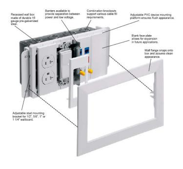
Spider's prewired drywall boxes, allows the contractor to reduce on-site labor costs and gives the client a low cost option for future expansion.
