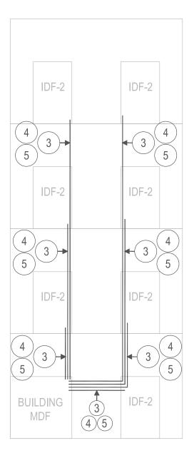
1 24-STR 50 MICRON OM3 MULTI-MODE/12-STR 9 MICRON SINGLE MODE FIBER
