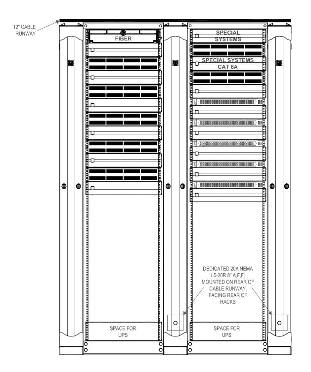
NOTE: 1. SPECIAL SYSTEM SECURITY, BMS, AV, CAMERAS, HVAC, FIRE ALARM, DIGITAL SIGNAGE 2. SPECIAL SYSTEM CAT 6A WAPS, UPLINK
